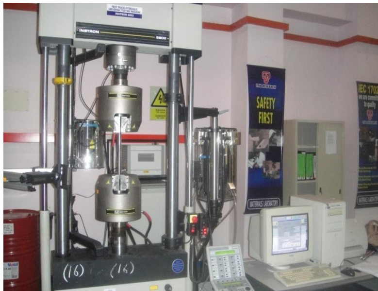
Figure 3. Fast Track Hydraulic Universal Testing Machine Instron 8802 of 250 kN load
