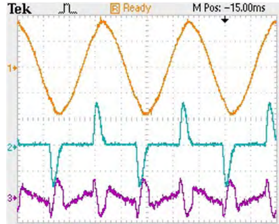
Fig. 22. Steady-state waveforms under a highly distorting load without using the HC: Ch1 denotes the output voltage (100 V/div), Ch2 denotes the load current (20 A/div), and Ch3 denotes the tracking error (10 V/div).
