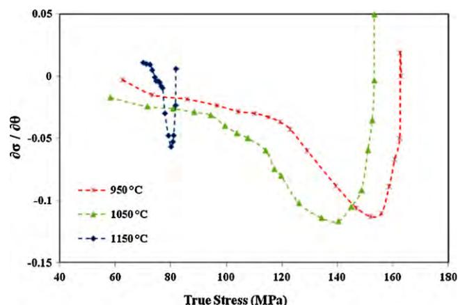
**Fig. 3.** The variation of hardening rate with flow stress at different temperatures; this has been utilized to estimate the  $\epsilon_C$  and  $\sigma_C$ .
