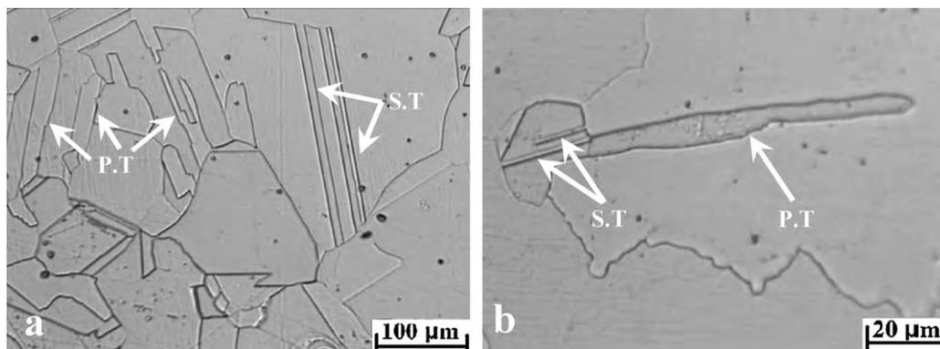
**Fig. 9.** The optical microstructure of the specimens deformed under  $10^{-1} \text{ s}^{-1}$  up to strain of 0.2: (a) after interpass time of 300 s at  $1150^\circ\text{C}$  and (b) after interpass time of 80 s at  $1050^\circ\text{C}$ .
