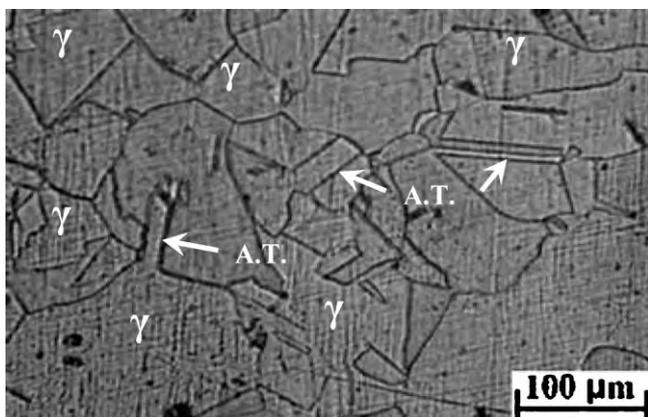
**Fig. 1.** Presence of annealing twins in the specimen annealed at 1100 °C for 45 min.
