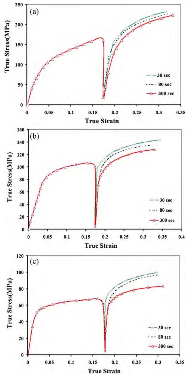
Fig. 5. The true stress–true strain curves of the experimental steel at strain rate of  $0.1s^{-1}$  and (a)  $950^\circ C$ , (b)  $1050^\circ C$  and (c)  $1150^\circ C$ .
