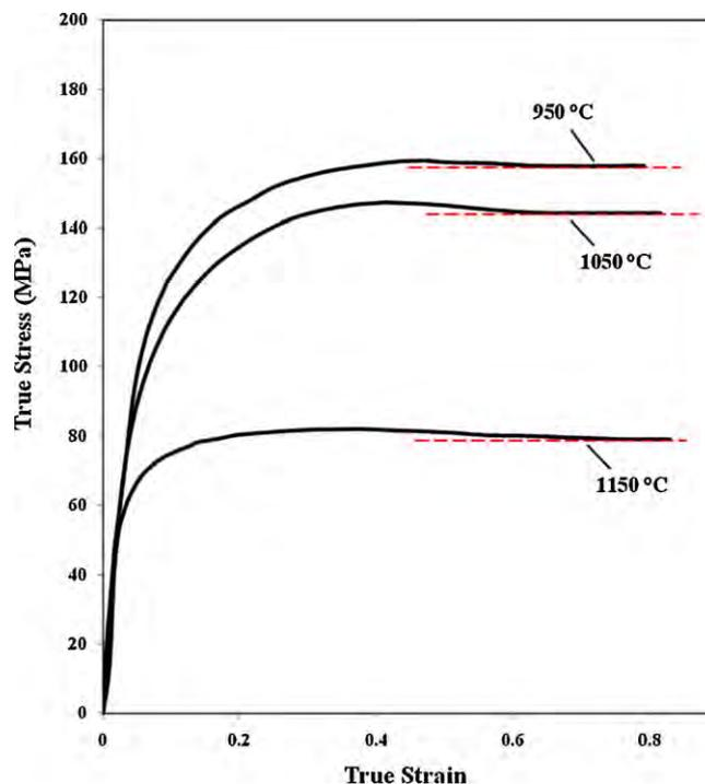
**Fig. 2.** The true stress–true strain curves of single-hit compression testing under strain rate of  $0.1 \text{ s}^{-1}$ .
