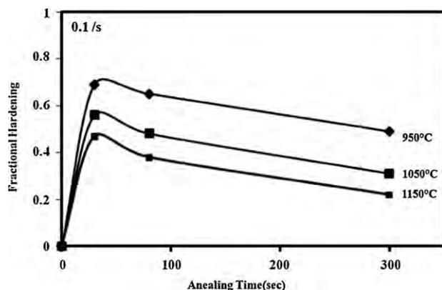
Fig. 6. The fractional hardening as a function of annealing time for various temperatures.
