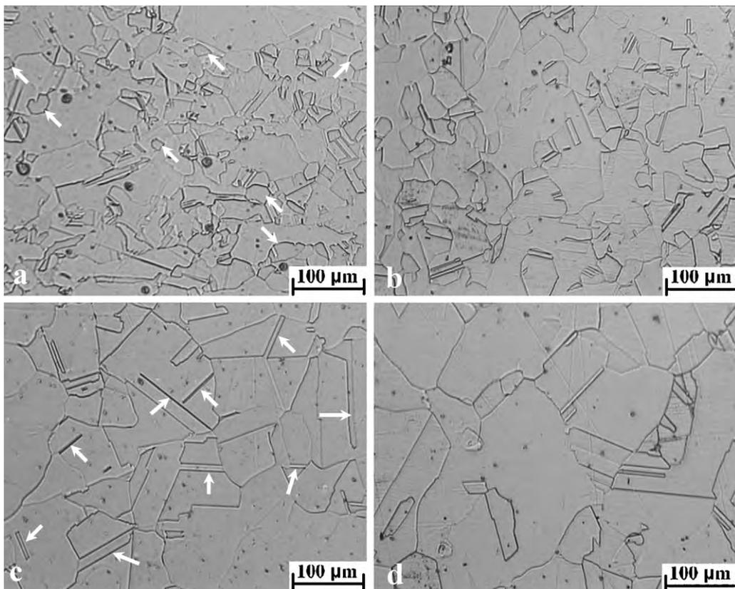
**Fig. 8.** The typical microstructures of the experimental steel interrupted and quenched after: (a) 80 s interpass time at  $950^\circ\text{C}$ , (b) 30 s interpass time at  $1150^\circ\text{C}$ , (c) 80 s interpass time at  $1150^\circ\text{C}$  and (d) 300 s interpass time at  $1150^\circ\text{C}$ .
