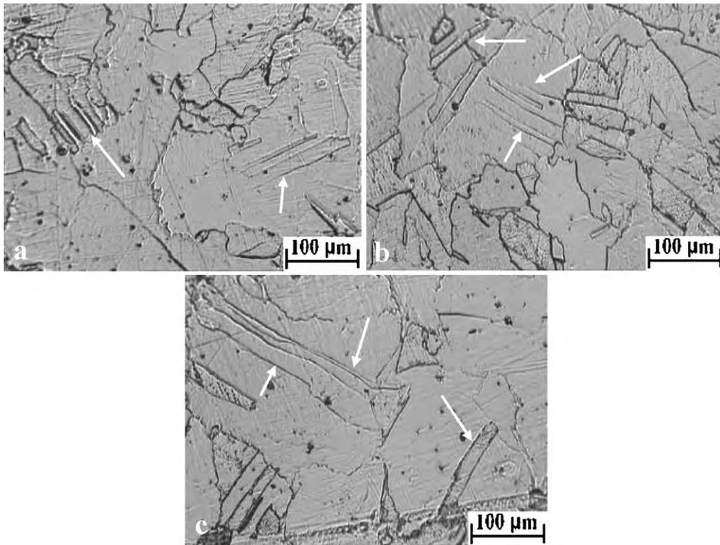
**Fig. 7.** The microstructures of the experimental steel right after applying the first deformation pass under strain rate of  $10^{-1} \text{ s}^{-1}$  and at temperatures of (a)  $950^\circ\text{C}$ , (b)  $1050^\circ\text{C}$  and (c)  $1150^\circ\text{C}$ .
