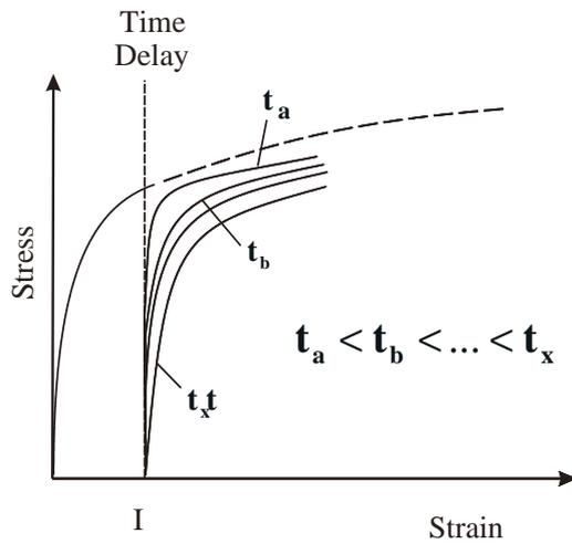
Fig. 4. A typical double hit flow stress with different interpass times.
