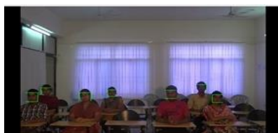
Fig. 10. Detection of seats – template matching Input Videos
