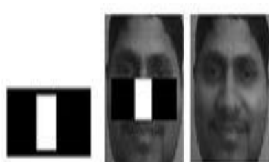
Fig. 4. Detection of nose using Haar features
