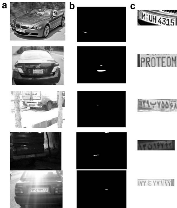
Fig. 19. Some result after applying match filter: column (a) car image, (b) detected regions, (c) detected plates.
