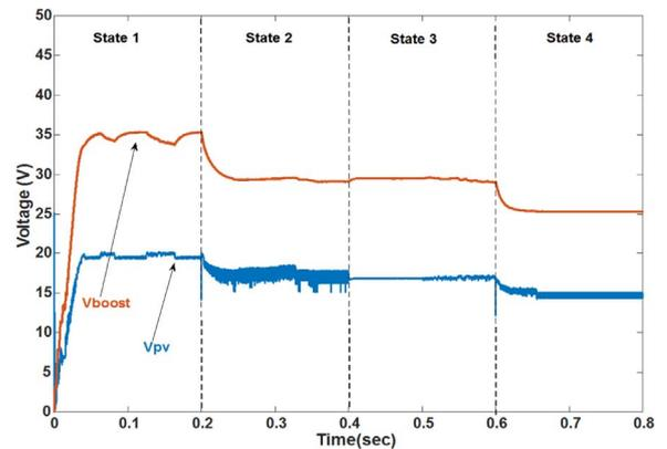
Fig. 17. The Voltage of PV panel and load of boost converter.
