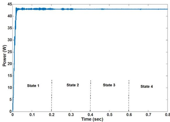
Fig. 21. The power regulated by PI control.
