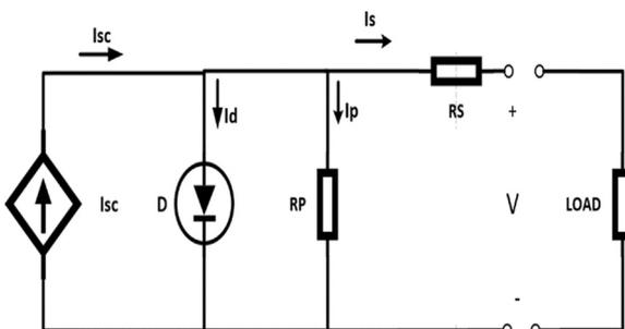
Fig. 2. Equivalent circuit of solar cell.
