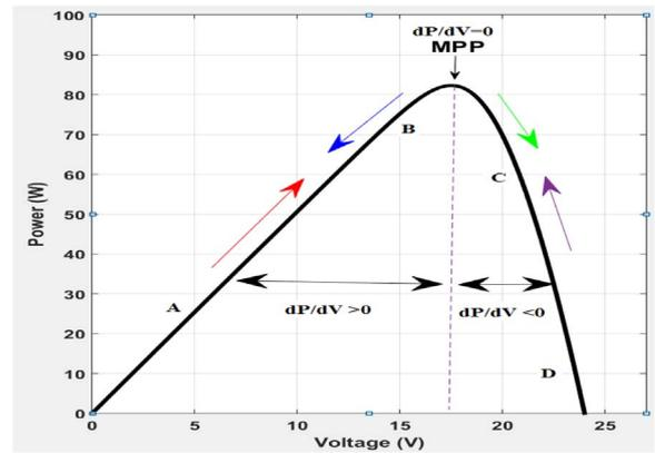
Fig. 5. P-V characteristic of PV panel for MPPT algorithm. (For interpretation of the references to color in this figure, the reader is referred to the web version of this article.)
