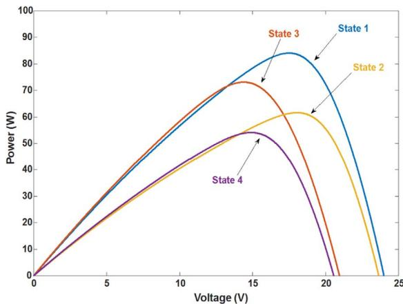
Fig. 15. The P-V curves under variable temperatures and irradiance.
