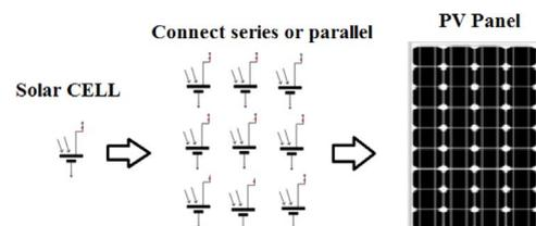
Fig. 3. From solar cell to PV panels.
