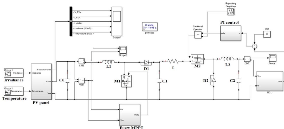
Fig. 22. The System constructed in Matlab/Simulink.
