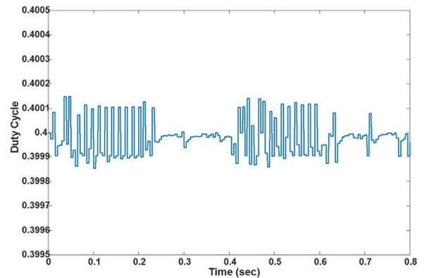
Fig. 18. The duty cycle regulated by FLC MPPT.
