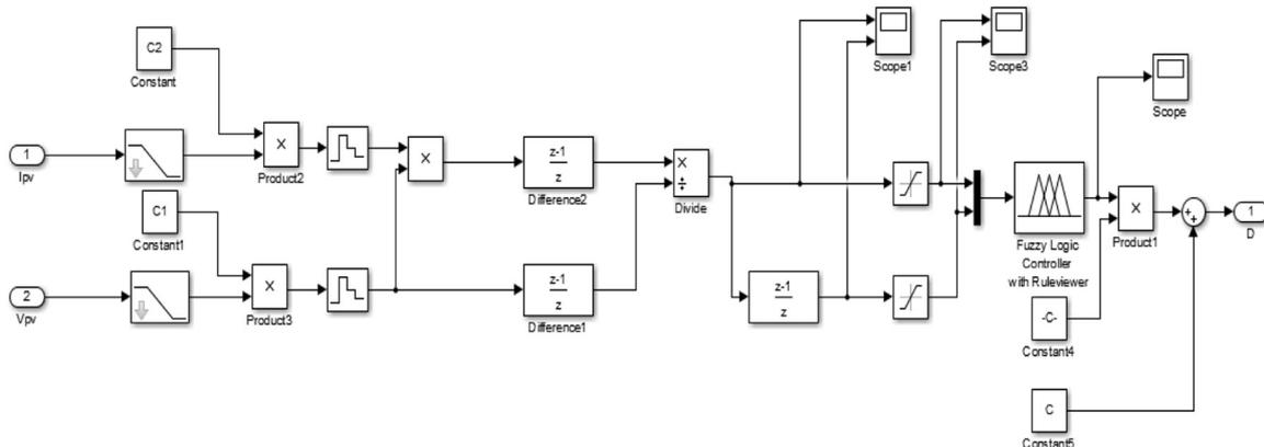
Fig. 8. The MPPT algorithm in Matlab/Simulink.
