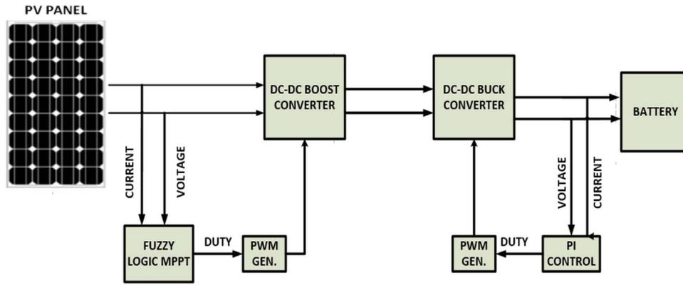
Fig. 1. PV system MPPT algorithm and PI control charge circuit.
