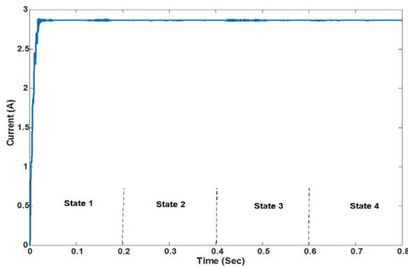
Fig. 20. The load current of buck converter.
