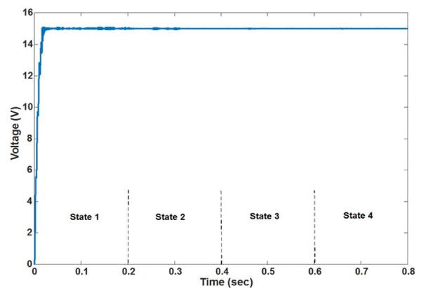
Fig. 19. The load voltage of buck converter.
