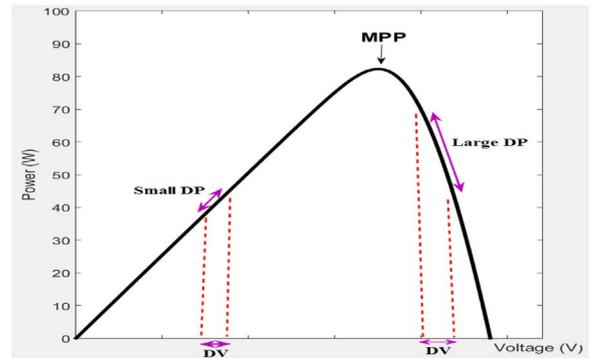
Fig. 6. P-V characteristic of PV panel for speed of MPPT.
