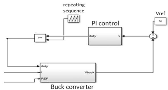
Fig. 12. PI control applied buck converter.
