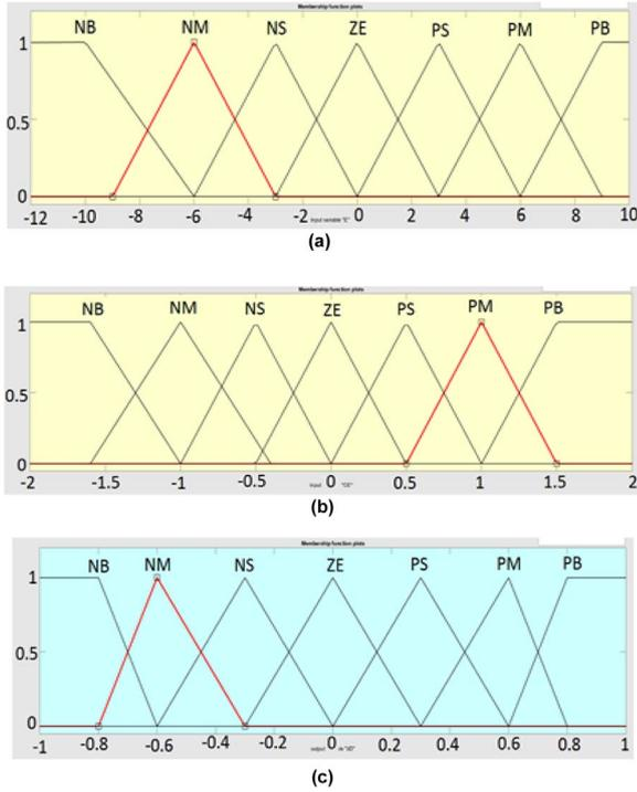
Fig. 7. (a) The input of FLC (Error, E), (b) The input of FLC (Change of error, CE) (c) The output of FLC (Duty, D).
