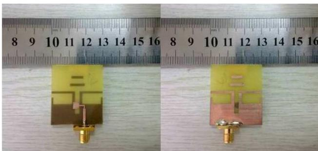
Fig. 7. Photographs of the fabricated antenna.
