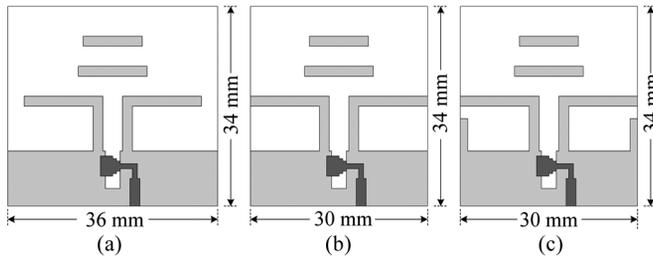
Fig. 2. Evolution of the ground plane of the printed quasi-Yagi Antenna, (a) Conventional printed quasi-Yagi antenna, (b) quasi-Yagi antenna with reduced ground plane, (c) quasi-Yagi antenna with modified reduced ground plane.
