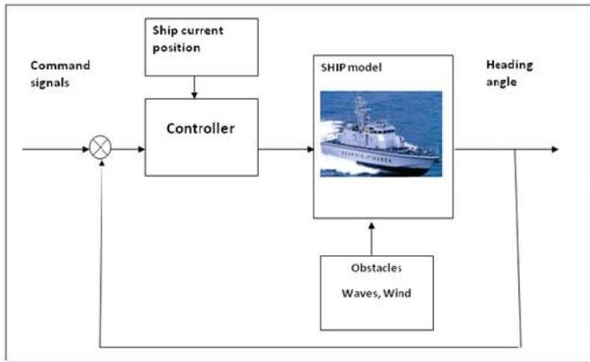
Figure 1: General simulation setup for ship tracking
