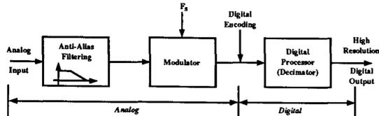
Figure 1 Application of the Mixed Analog Digital Compiler for the Compilation of an Oversampled A/D Converter
