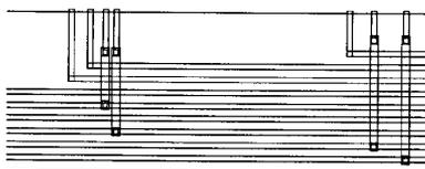
Figure 11 Details of the Balanced Differential Signal Routing
