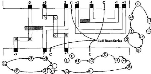
Figure 4 Balanced Differential Signal Routing and the two Constraint Graphs showing a Subset of Their Edges
