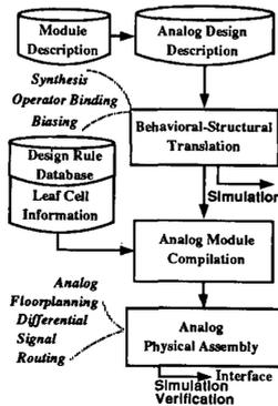
Figure 3 Details of the Analog Subsystem Architecture
