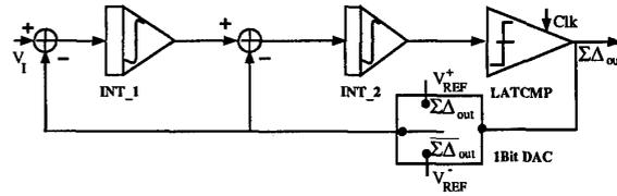
Figure 7 Simplified Block Diagram of a 2nd Order Oversampled A/D Converter
