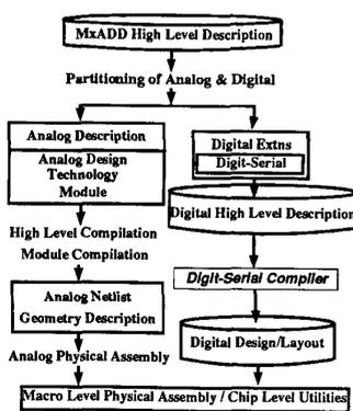
Figure 2 System Architecture of the Mixed Analog Digital Compiler
