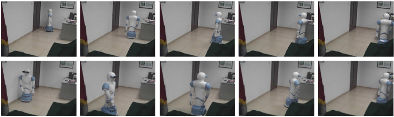
Fig. 9. Scenes of SIAT mobile robot performing wall-following navigation in an indoor experiment.
