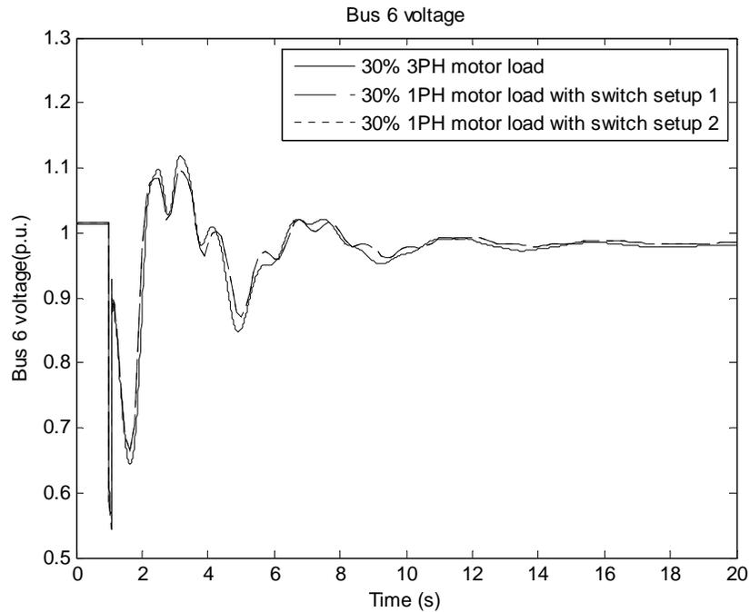
Figure 6-14 Bus 6 voltage magnitude for 30% motor load
