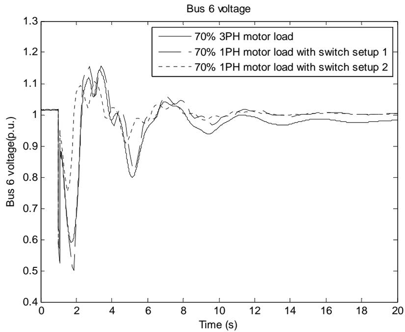
Figure 6-18 Bus 6 voltage magnitude for 70% motor load
