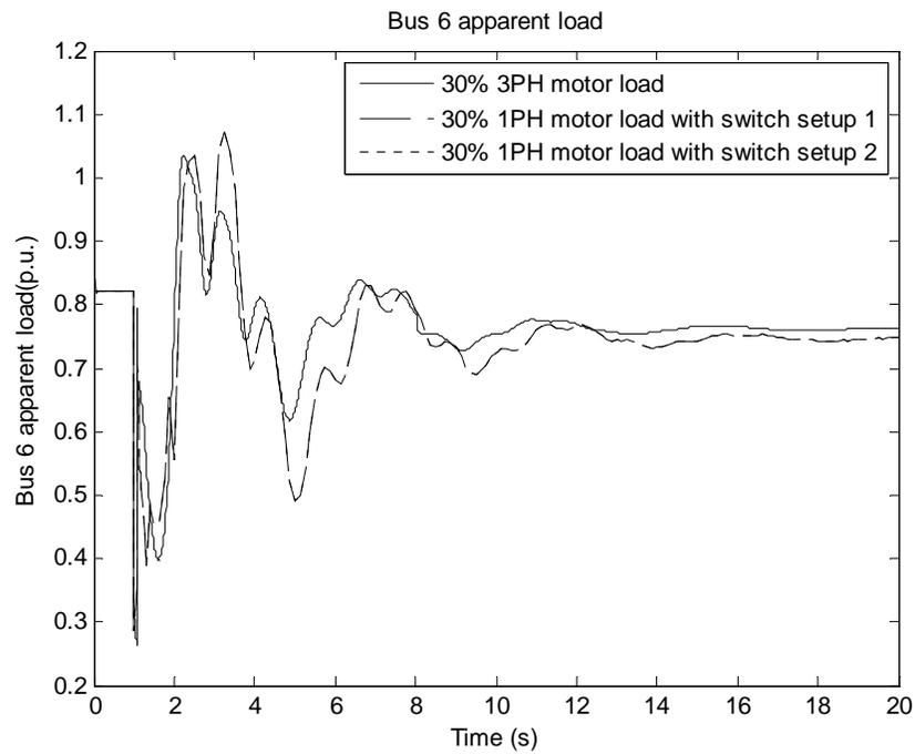
Figure 6-13 Bus 6 load for 30% motor load
