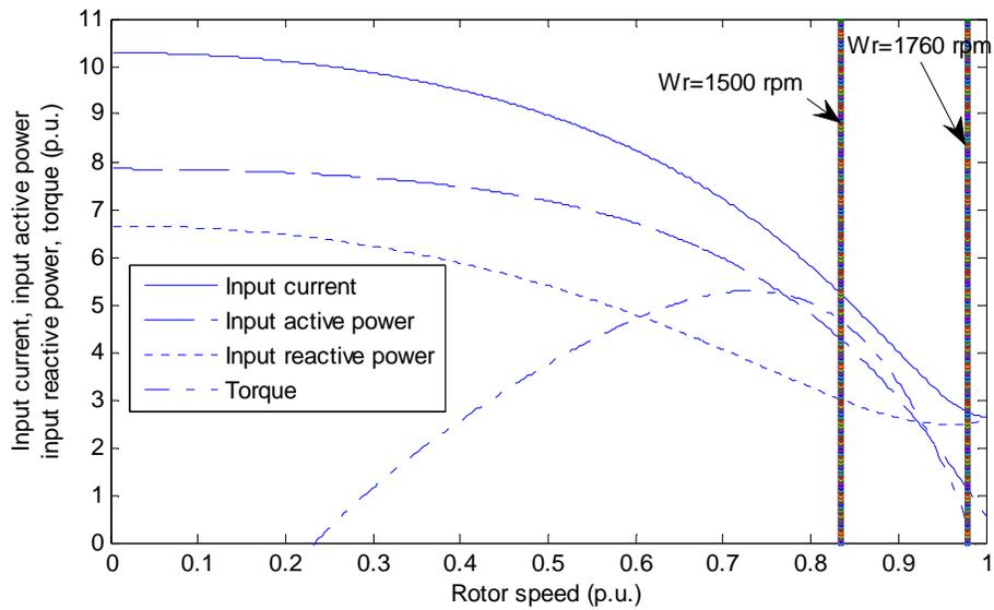
Figure 3-4 General characteristics of the single-phase induction motor
