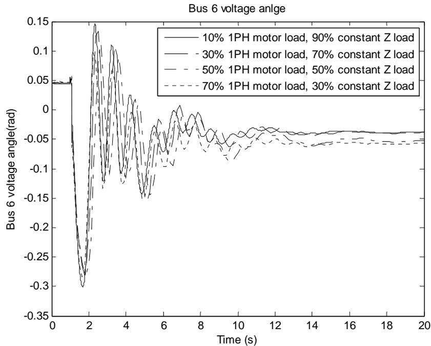
Figure 6-10 Bus 6 voltage angle with protection setup 2
