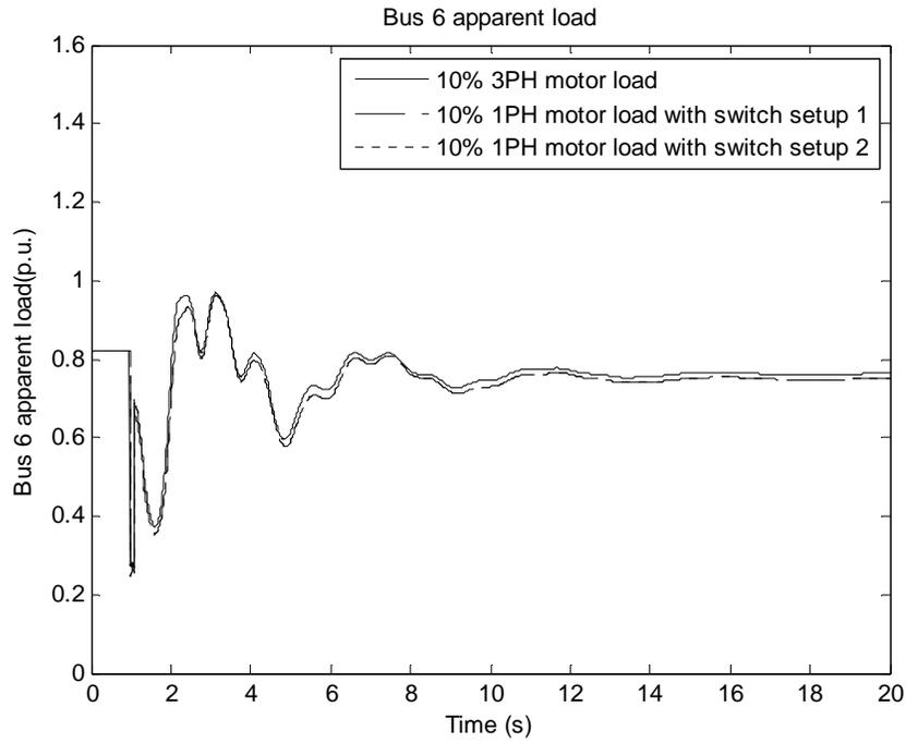
Figure 6-11 Bus 6 load apparent power for 10% motor load
