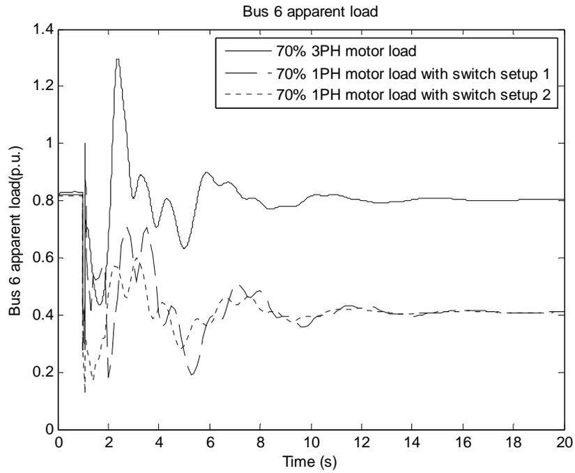
Figure 6-17 Bus 6 load for 70% motor load
