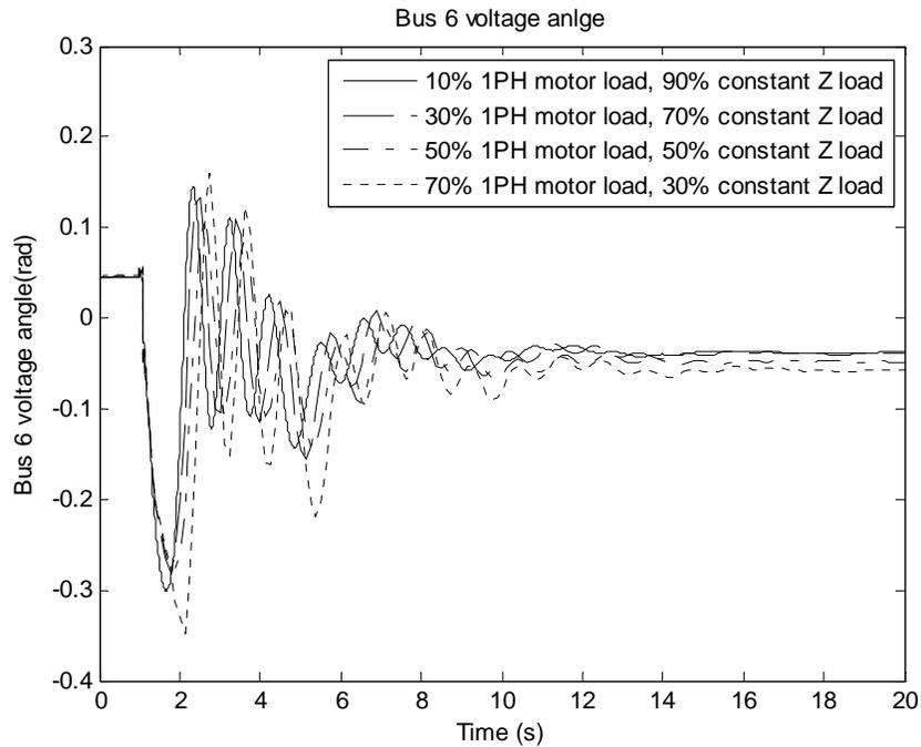
Figure 6-7 Bus 6 voltage angle with protection setup 1
