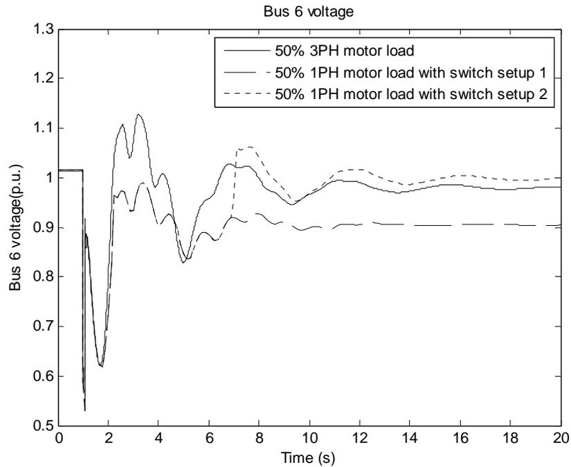
Figure 6-16 Bus 6 voltage magnitude for 50% motor load
