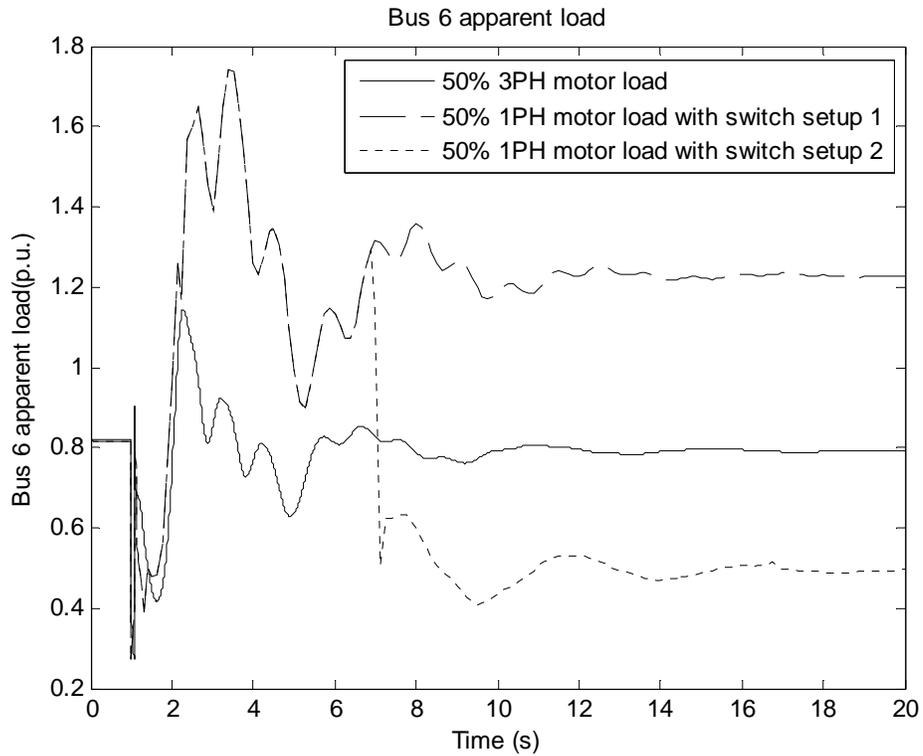
Figure 6-15 Bus 6 load for 50% motor load
