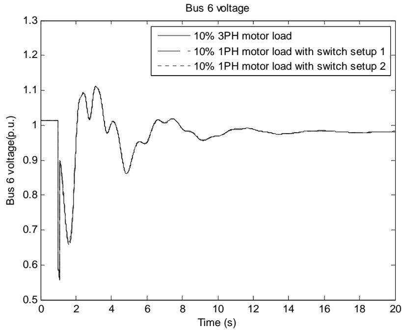
Figure 6-12 Bus 6 voltage magnitude for 10% motor load
