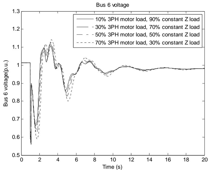
Figure 6-3 Bus 6 voltage magnitude for three-phase motor load
