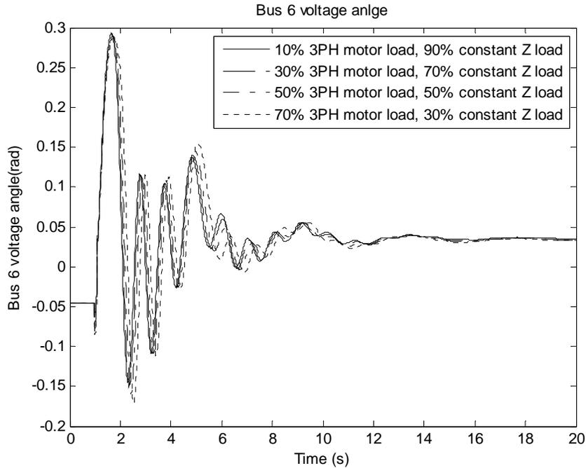
Figure 6-4 Bus 6 voltage angle for three-phase motor load
