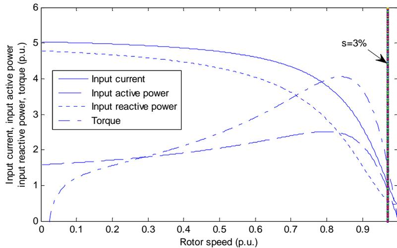
Figure 3-2 General characteristics of the three-phase induction motor
