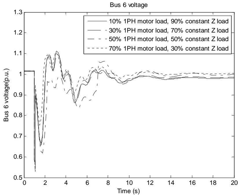
Figure 6-9 Bus 6 voltage magnitude with protection setup 2
