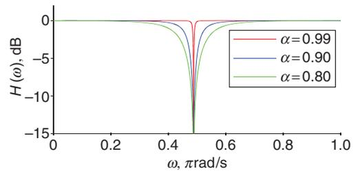
Fig. 2 Amplitude response of notch filter for different  $\alpha$
