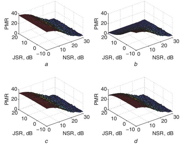
**Fig. 4** PMR test of anti-jamming schemes for  $\alpha = 0.99$  and  $M = 8$
