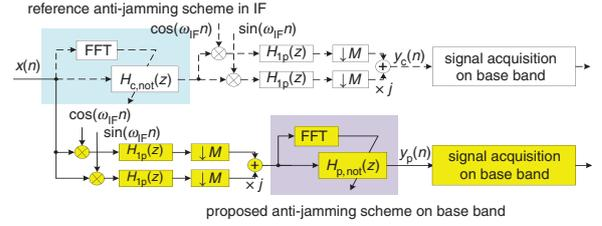
Fig. 1 Comparison of reference scheme and proposed scheme
