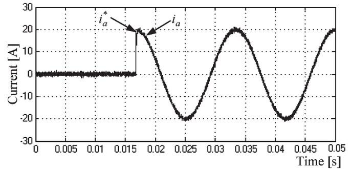
Fig. 6. Performance of the proposed deadbeat current controller implemented in fully digital system.
