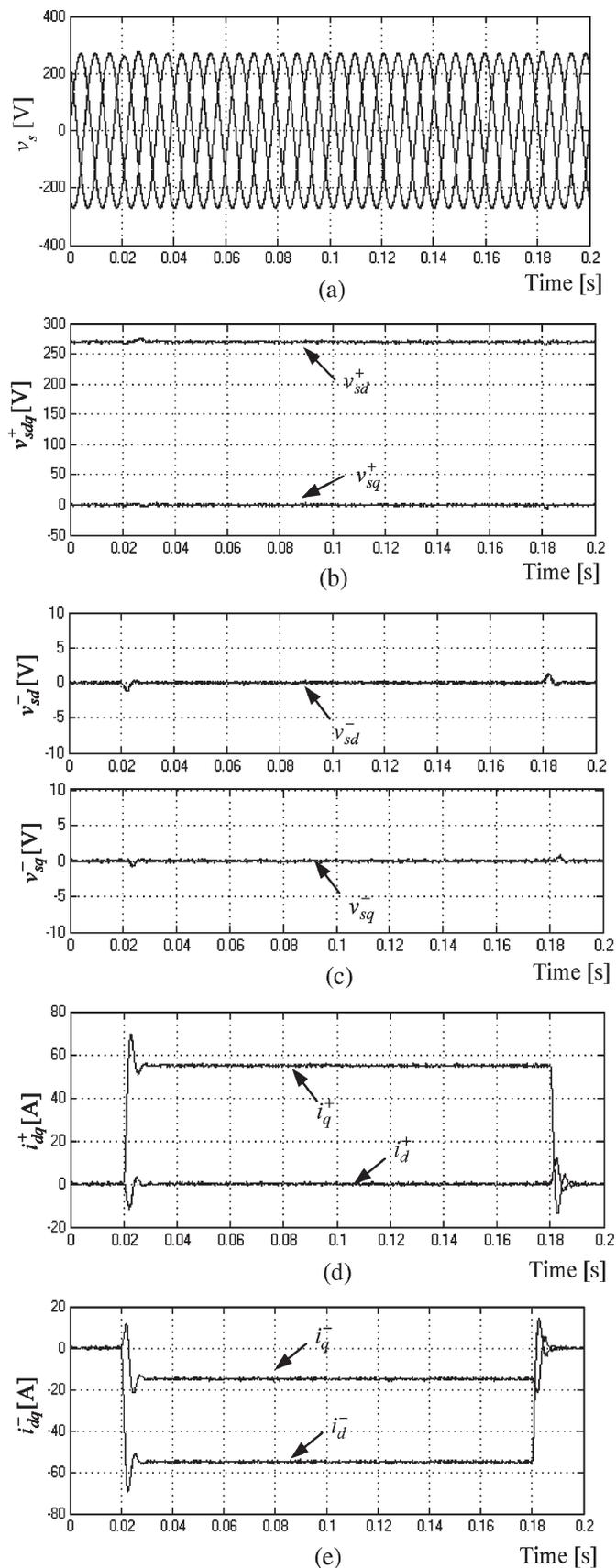
Fig. 13. Control performance of the proposed scheme during unbalanced voltage disturbance. (a) Voltage waveforms. (b) and (c) Positive- and negative-sequence  $dq$  components of the grid voltage. (d) and (e) Positive- and negative-sequence  $dq$  components of the injected currents.
