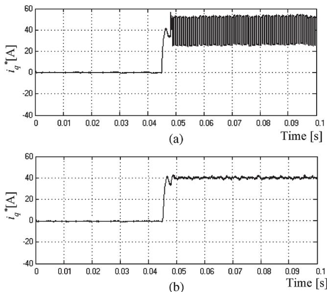
Fig. 14. Control effort of the proposed voltage controller (a) with a hard switching function and (b) with switching-function approximation.
