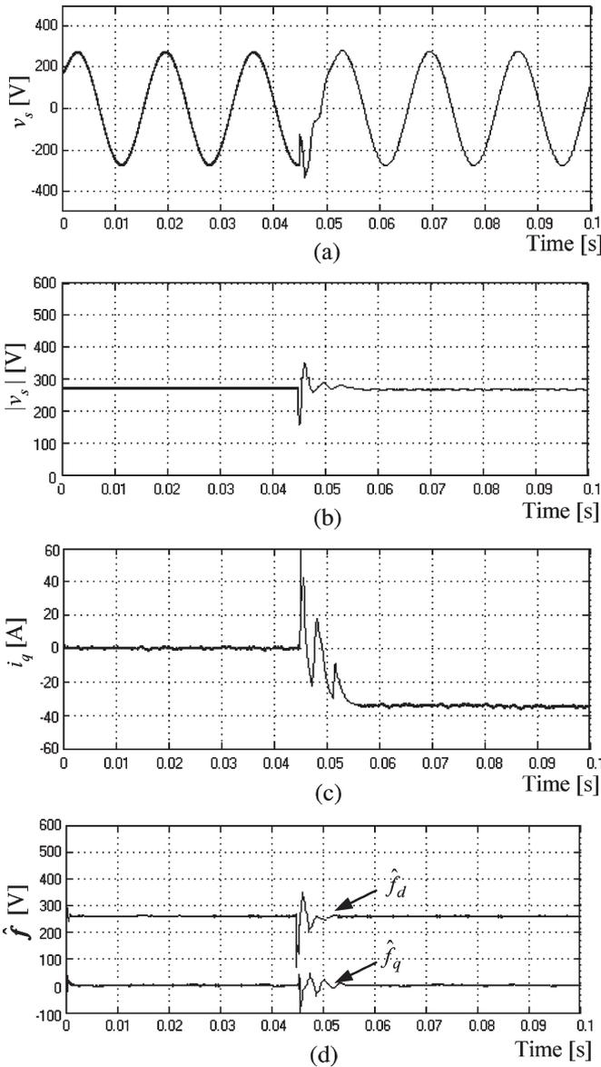
Fig. 11. Disturbance rejection performance with the proposed controller against voltage transients initiated by capacitor switching. (a) Voltage waveform. (b) Voltage magnitude at the PCC. (c) Reactive current injected. (d) Estimated uncertainty function.
