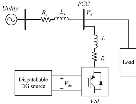
Fig. 1. Network connection of a VSI with DG.
