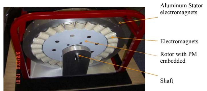
Fig. 5. Prototype of the PMSR machine
