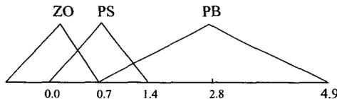
**Fig. 3 Membership function of  $\Delta\omega$  (rad/sec)**
